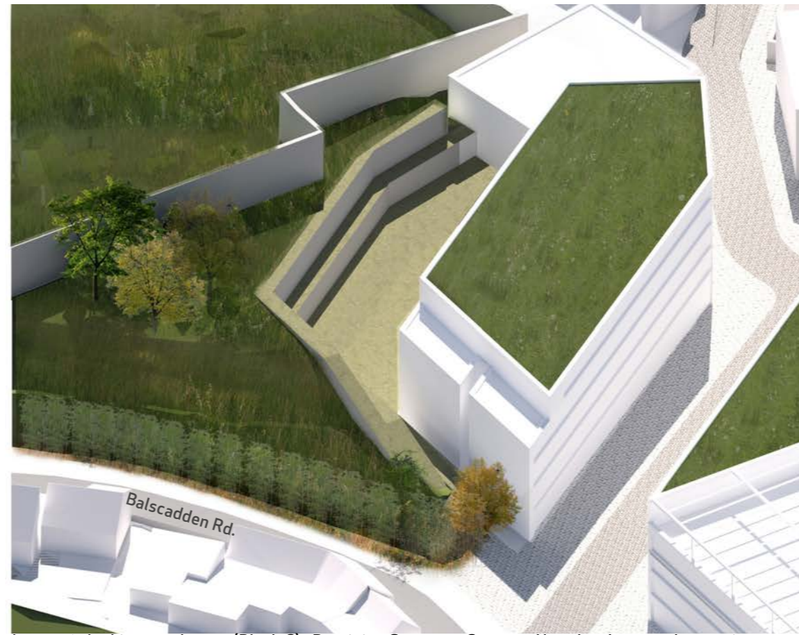
Isometric looking south west (Block C) . Retaining Structure Concept: New development buttressing retaining walls.
